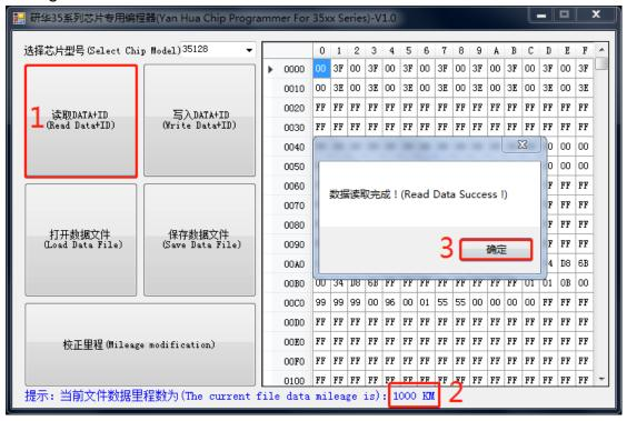
14.If the displayed mileage is the same as what you want, cut off the handle of the Simulator, and solder the Simulator to the original EEPROM
