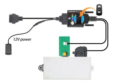
Step 1: Connect the CAS2/CAS3, CAS3+ CAS3++ modules according to the connection diagram.
