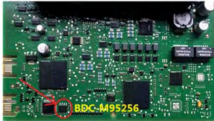
Picture 2: EEPROM position on BDC System
