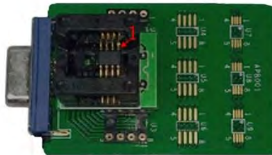
Picture 4: Pin 1 position on the clamp
