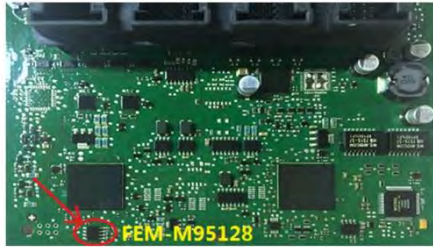
Picture 1: EEPROM position on FEM System
