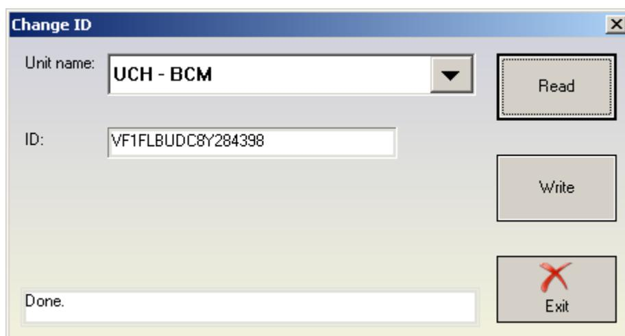
For each device you can try to read and change the Vehicle Identification Number. When changing this number there is also a checksum which is calculated automatically.
