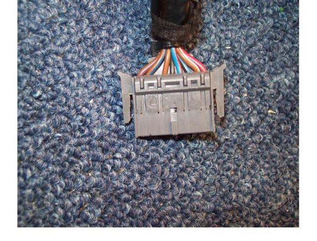
Connecting emulator in place of a original immobilizer in the ignition switch.
