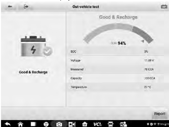
Figure 7-9 Sample Out-vehicle Test Results Screen
