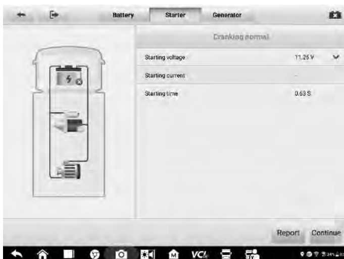
Figure 7-6 Sample Starter Test Result Screen
