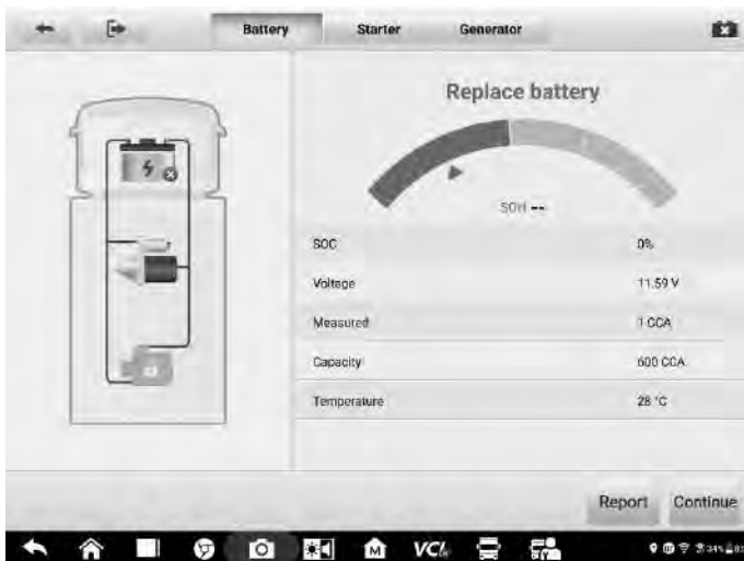
Figure 7-5 Sample Battery Test Results Screen
