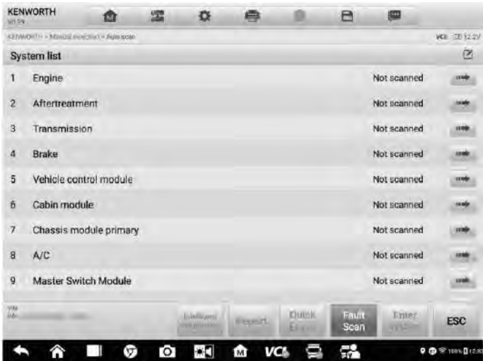
Figure 5-4 Sample Fault Scan on System List Screen 1
