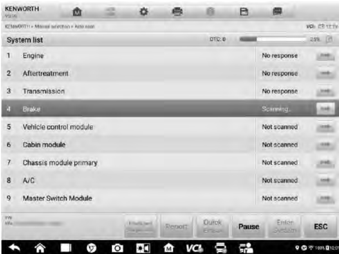
Figure 5-5 Sample Fault Scan on System List Screen 2
