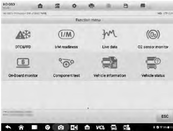
Figure 4-27 Sample OBDII Diagnostic Menu
