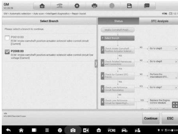
Figure 5-22 Sample Repair Assist Screen 3
