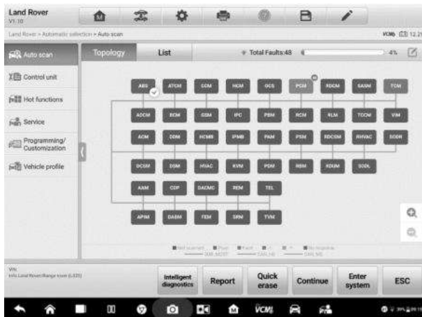
Figure 5-6 Sample Fault Scan on Topology Screen
