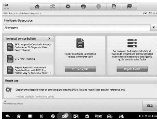
Figure 5-20 Sample Repair Assist Screen 1
