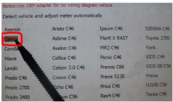
7, show "C46" as follows, it indicates to remove the Instrument and to find C46 chip. Note: the same as to the other cars models, when it displays chip model, just to remove the Instrument and find the corresponding chip model.
