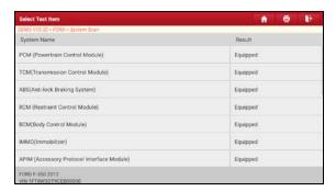
Tap the desired system to go to the diagnostic function selection screen. For detailed operations on diagnostic function, please refer to Chapter 6.2.3.
