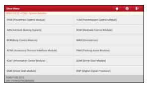
Swipe the screen from the bottom to view the vehicle system on the next page. Tap the target system (take **ECM** for example) to navigate to the diagnostic function selection screen.
