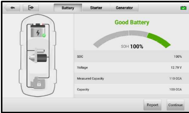
Figure 10-7 Battery Test Results Screen
