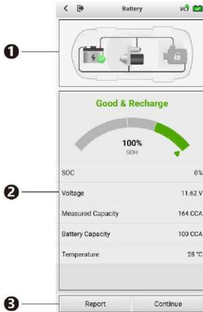
Figure 4-7 Sample Battery Test Result Screen
