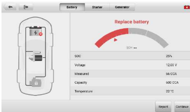
Figure 8-7 Battery Result Screen
