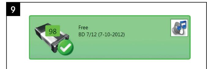
If configuration is successful, a green tile with the number of the XENTRY Connect will be displayed. You can now use the devices: Remove the black Ethernet connecting cable to work via WLAN and with an online connection. Then click on the green tile in order to read out the data for ordering the StartKey.
