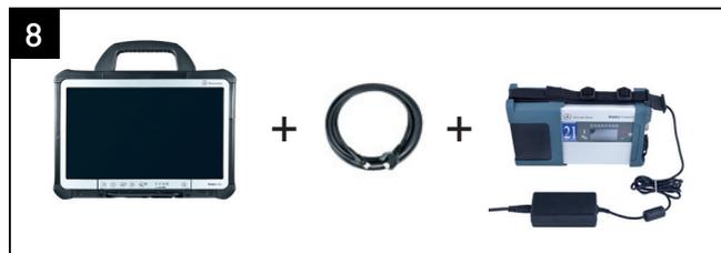
In the final steps, the configuration is transferred from the XENTRY Tab/XENTRY Tab 2 to the XENTRY Connect. You will be prompted to interconnect the devices using the supplied black Ethernet connecting cable. This cable connection is required only for configuration, not for operating the XENTRY Kit/XENTRY Kit 2.
