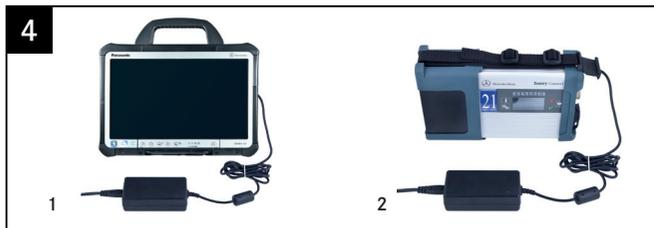
Completely charge both devices and turn on the XENTRY Connect. Starting the XENTRY Connect for the first time can take up to 10 minutes. Configuration can be started whilst both devices are still charging. **Attention!** Be sure to use the correct power supply units!
