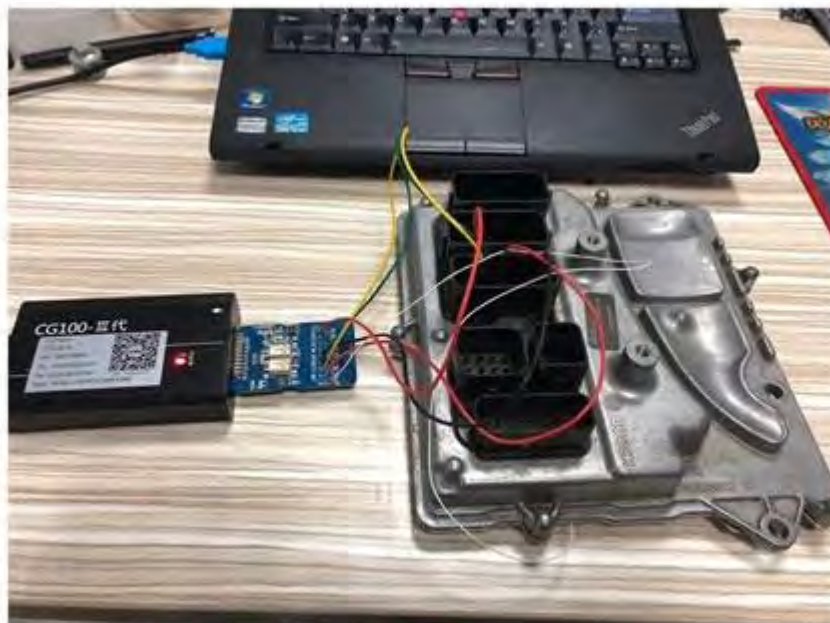
Engine module wiring
